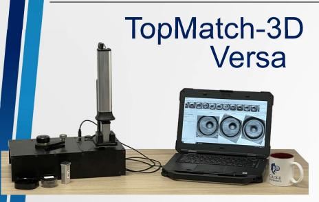
Introducing the latest addition to Cadre's courtroom-proven VCM platform - the newly redesigned Versa Scanner. The Cadre TopMatch-Versa system uses the same gel technology as our validated desktop system to rapidly capture high-resolution, 3D surface topographies. With a lateral spacing interval of approximately 2.75 microns per pixel, the Versa scanning unit provides accurate measurements which can be analyzed using the same TopMatch software as our desktop system
